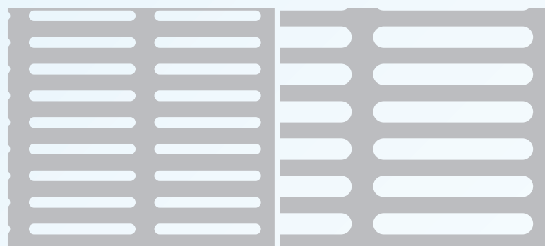
2x20 p. 5x23,5 v/p 34% 4x30 p. 7x34 v/p 49% 15x45 p. 21x50 v/p 60%
